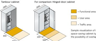
Sample visualization of the functional floor space required by space-saving cabinet types (The example does not take into account the possibility of overlapping traffic areas according to regulations)
